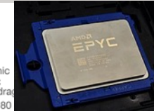
2019 AMD Epyc – 32,000,000,000 transistors
